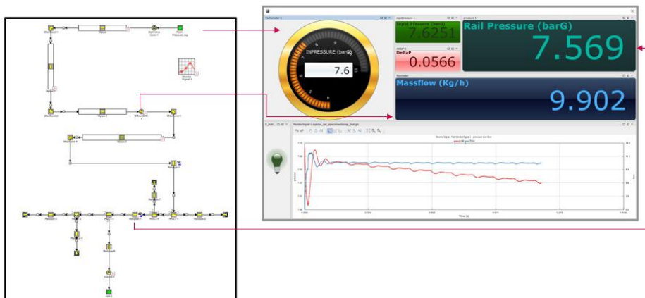
Figure 2.40 Optimized Model of the Nozzle, Rail assembly and Pipe connections Fig. Real time dashboard created to easy analysis of run time data and compare while test bench is running in parallel
